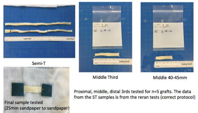
Figure 2 A description of the cutting process used to make the proper sized samples for the ST and GR.
