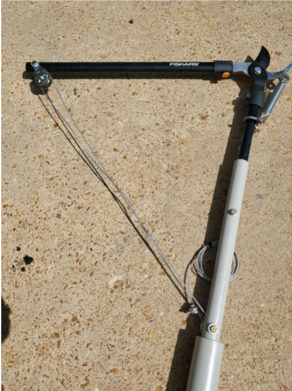
Figure 20: Shears mounted on pole
