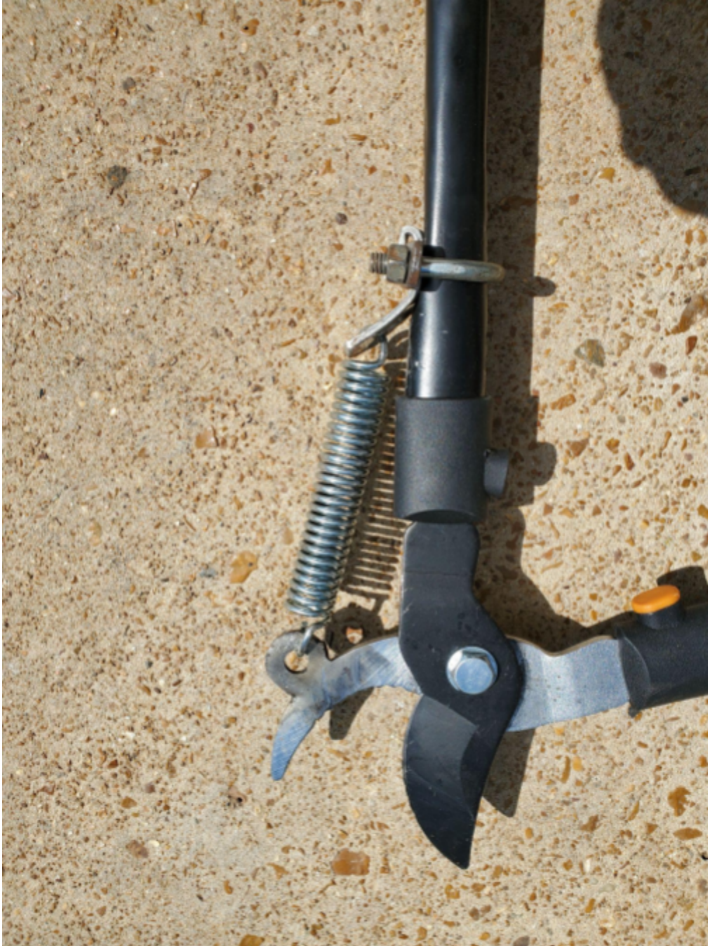
Figure 21: Close up of shear blades and compression spring
