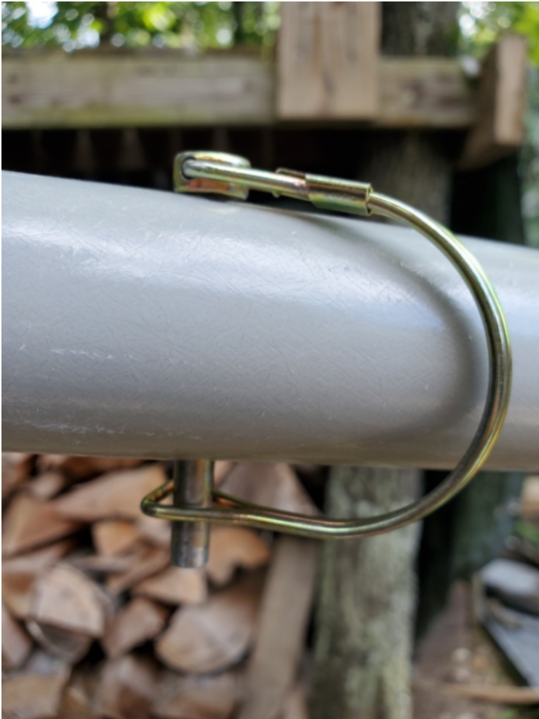
Figure 23: Close up of PTO pin going through pole
