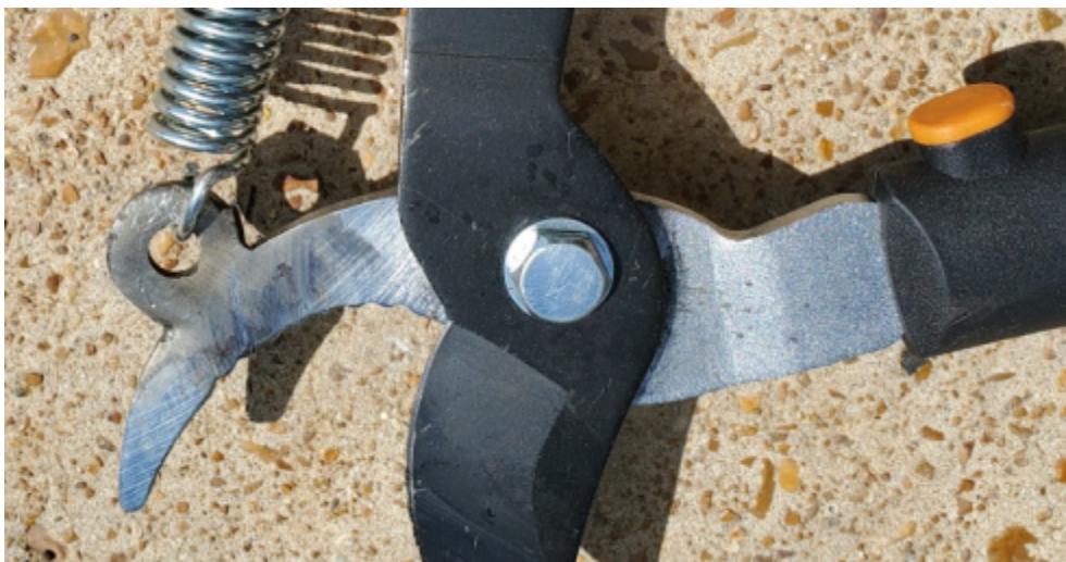
Figure 35: Close view of lopper hood and welded washer
