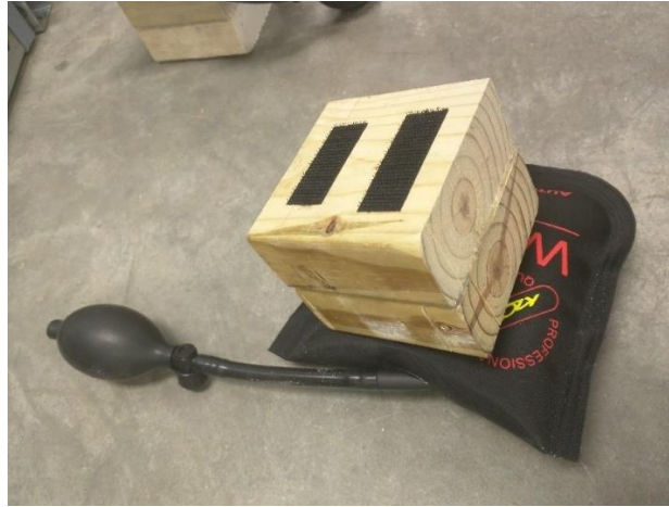
Figure 20. Wood padding - Air wedge
