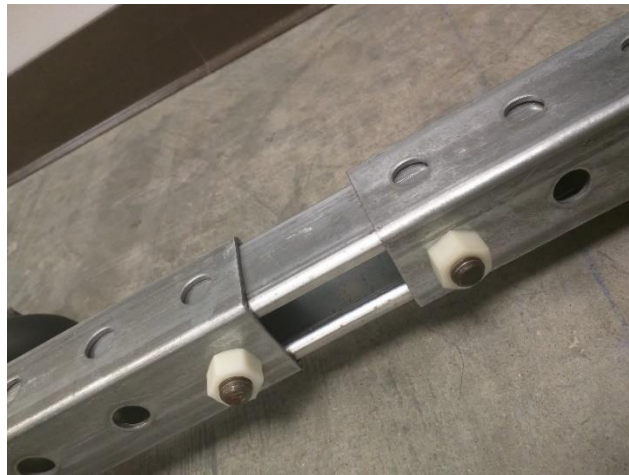
Figure 21. Sliding arms and pins
