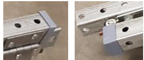
Figure 12. Added 3D printed caps
