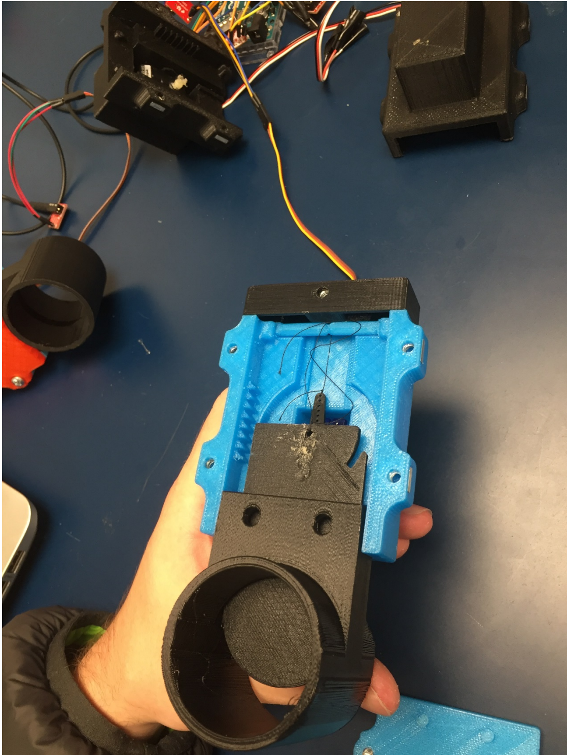
Figure 21: The inside of the motor housing, showing the door and motor subassembly. The door is connected to the motor arm using thread that is looped over a shaft. The thread is tied to both the door and the motor arm.
