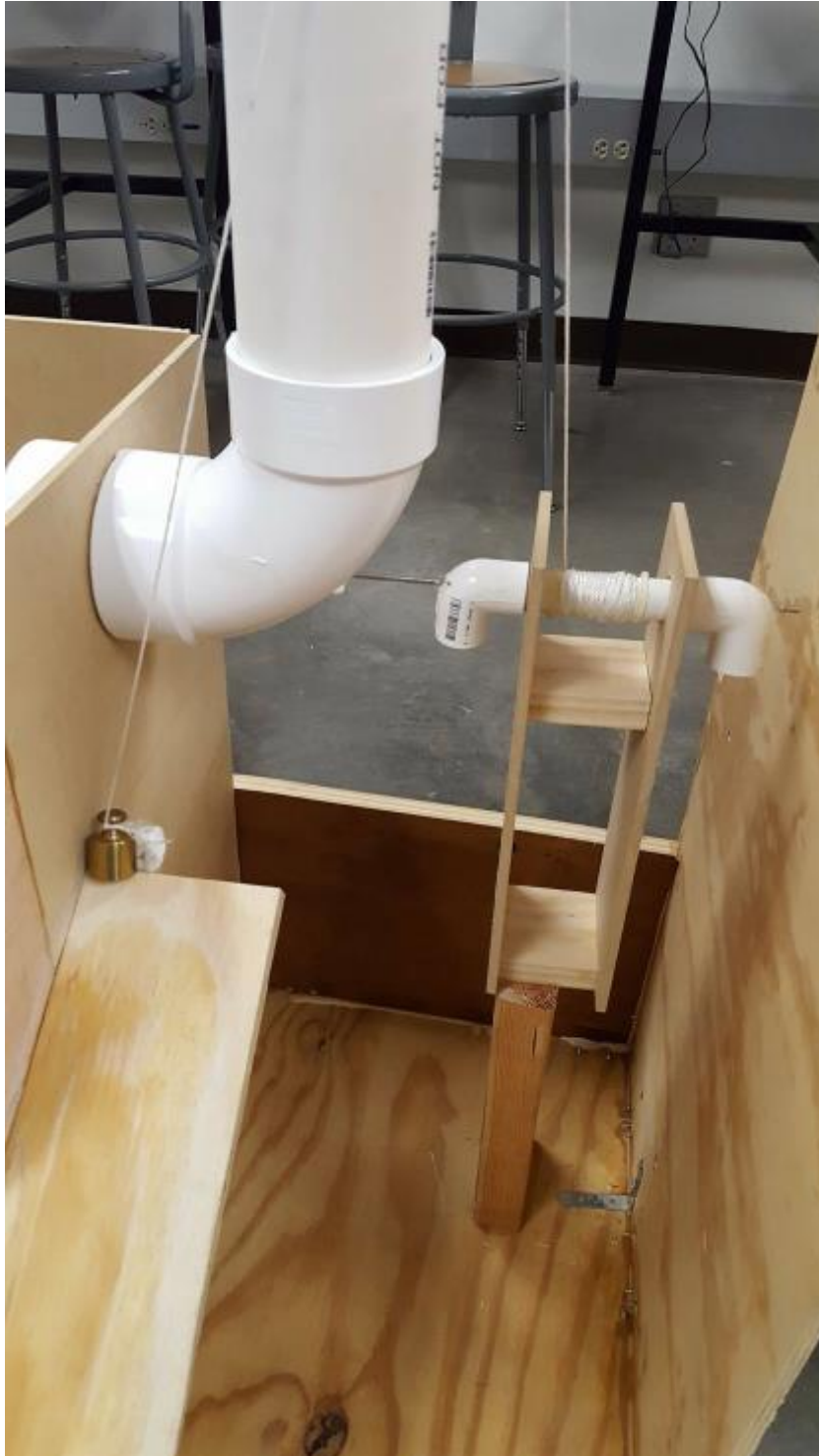
Figure 28: Picture of fan rotational mechanism attached to a pulley and weight.
