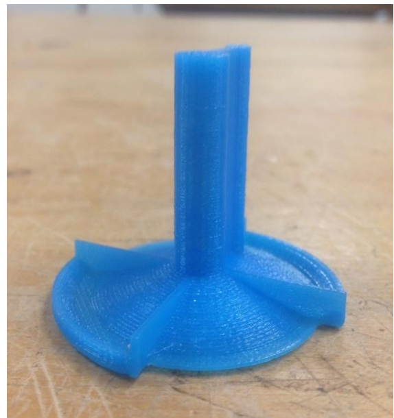
Fig 27 One of the redesigned deflectors. The raised lips are shown in this image. The height of these lips will likely need to be increased to get the desired performance.
