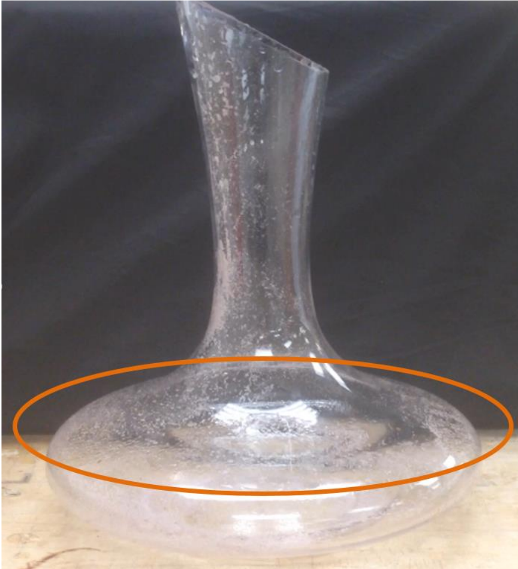
Fig. 23 The hardest area for the current brush to reach is outlined in orange. Some debris can still be seen on this portion of the decanter
