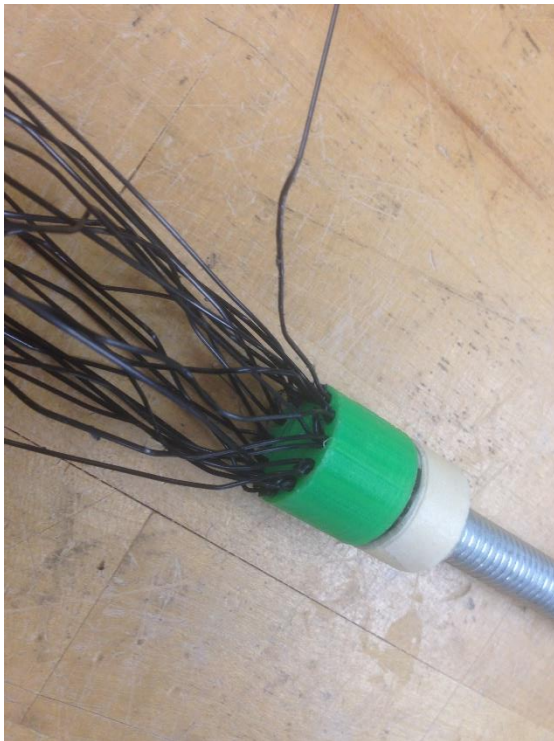
Fig. 26 The first prototypes filaments were hand threaded through our brush head.
