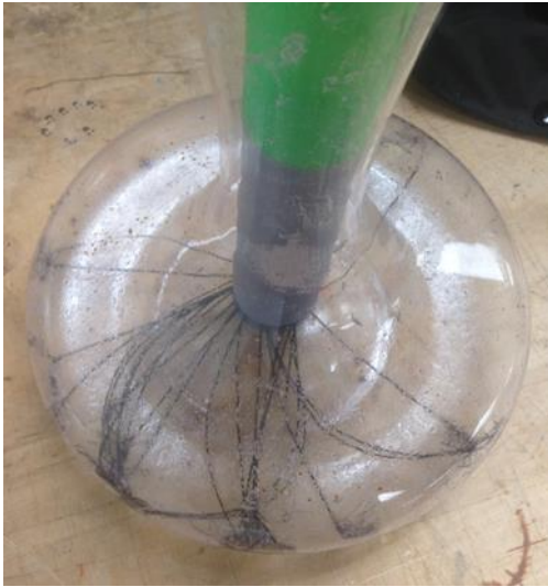
Fig 24 This image shows the first prototype brush extended within our test vessel. The bristles easily reach the outer edge of the test vessel.
