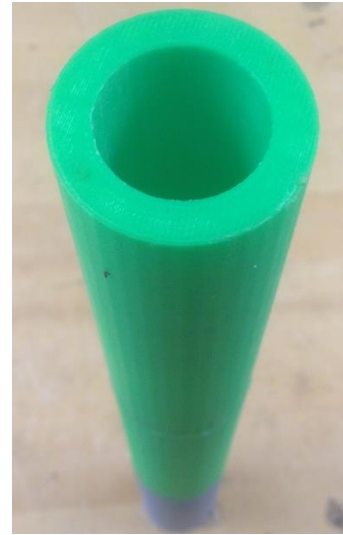
Fig. 25 Decreasing the difference between the inner and outer diameters of the sleeve will allow us to greatly reduce the overall size of our brush.
