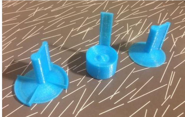
Fig. 23A The three redesigned deflector are picture here. The middle deflector will be used with a redesigned outer sleeve, while the other two fit into our first prototype's outer sleeve.
