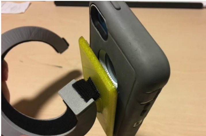
Figure 24: Velcro Holding Carriage at End-Cap
