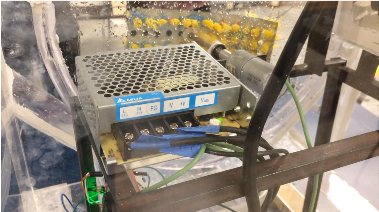
Figure 21 Power supply for pump, motor, and Arduino
