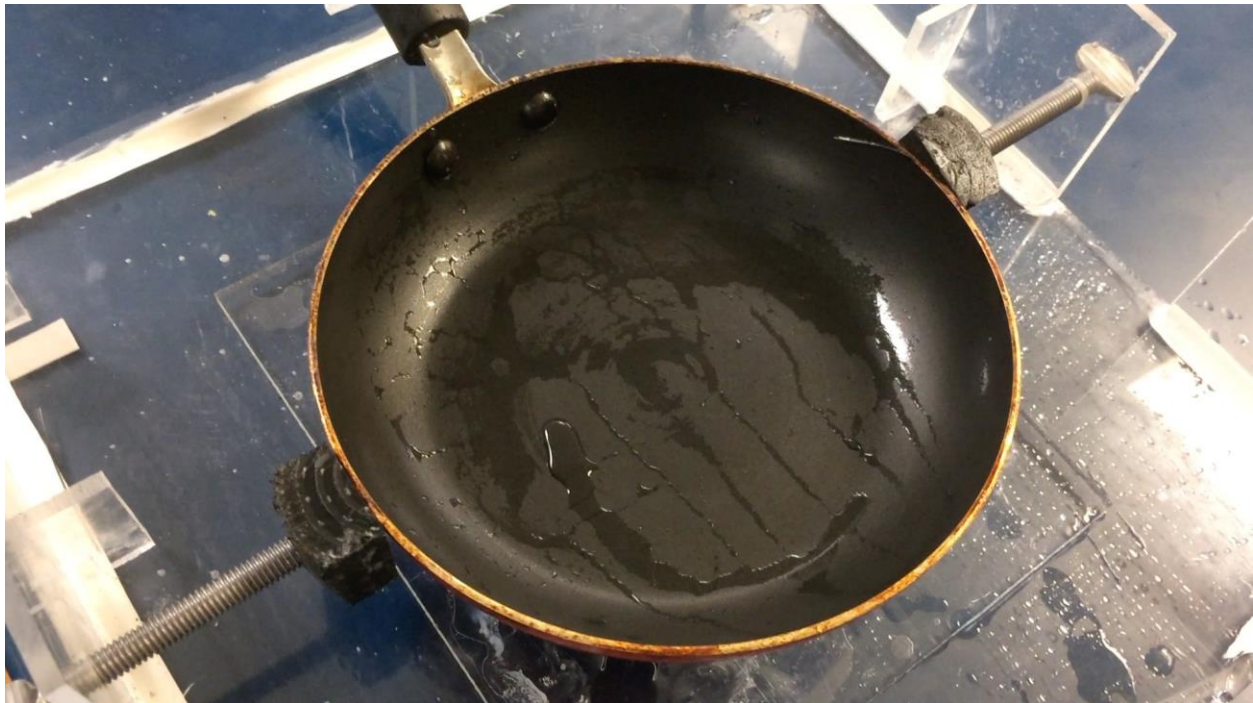
Figure 22 Mechanism for keeping pan secured
