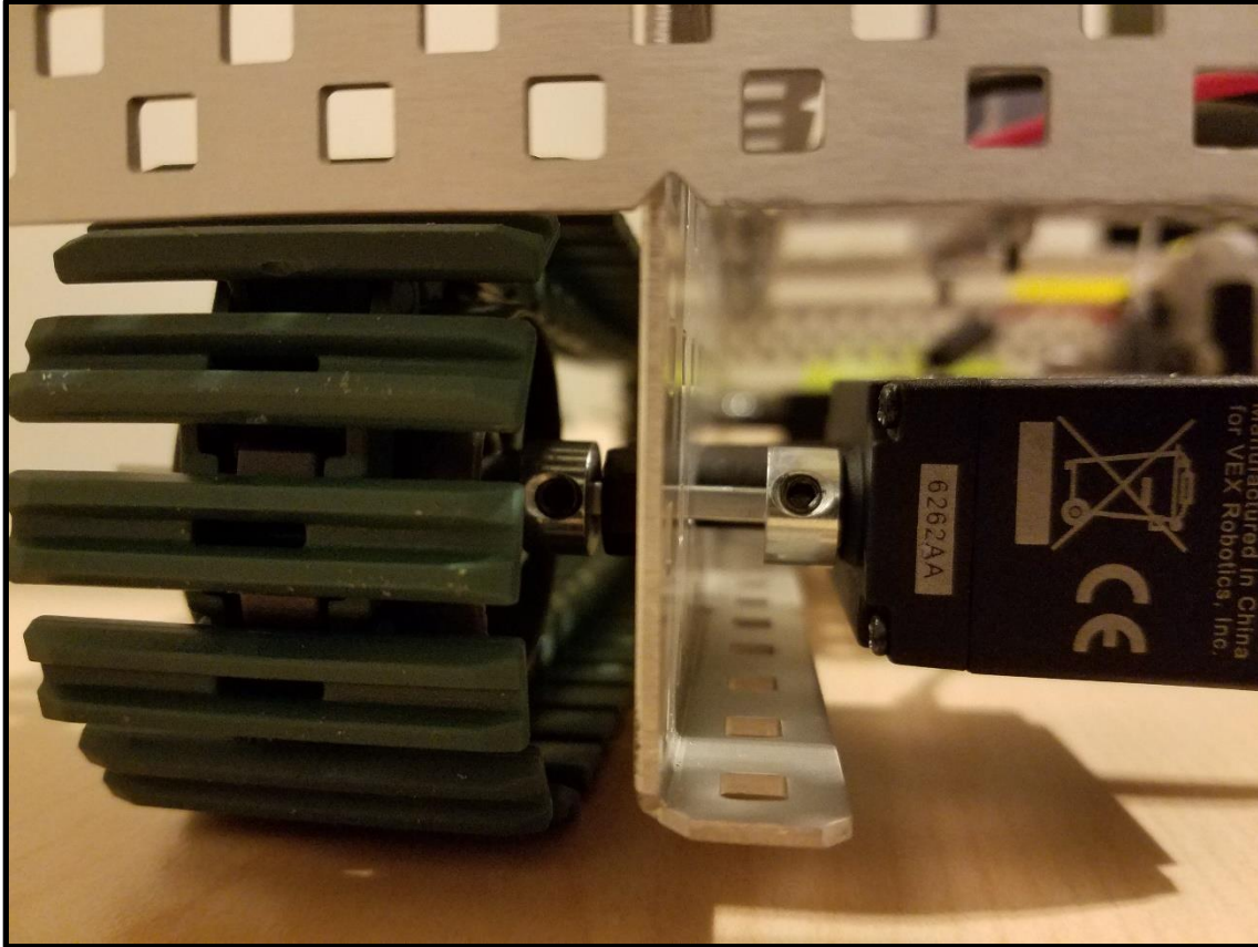
Fig. 28 This picture displays the connection between one of the four motors that power the tank treads and the tank treads. It is a square shaft that fits into the motor followed by a set of collars to keep the shaft from coming out of the motor. The square shaft has another female connection on the tank tread wheels fitting nice and secure.
