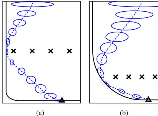
Figure 1: 2D navigation. **(a)** The robot (dashed blue line) localizes itself by approaching the wall (black) while avoiding the obstacles (X) and reaching the target (triangle). Blue ellipses depict the covariance. **(b)** An optimal solution that interacts with the curved part of the constraint manifold.
