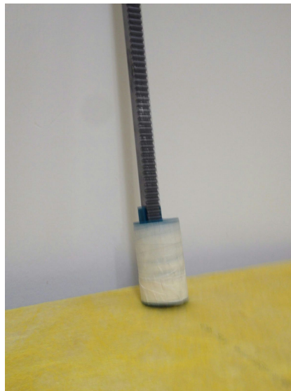
Figure 32: Crusher Rack and Head
