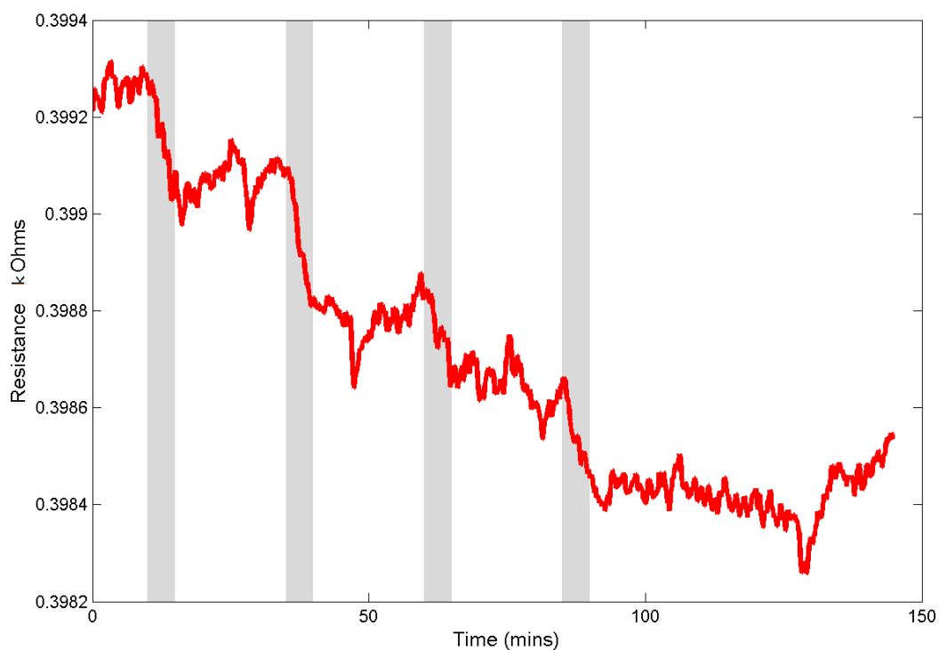
Figure. 8 Resistance vs. Time under hexane exposure, concentration 2.5 ppm
