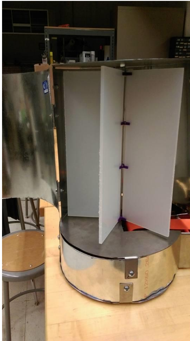
Figure 6: The door open for the empty petri dishes to be inserted before the process begins both up close (above) and at a distance (below, Figure 5) to see how the parts interact.
