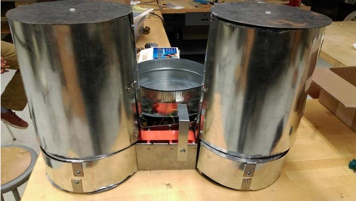
Figure 4: The assembly of all parts of the machine interconnected for use in pouring petri dishes. (above)
