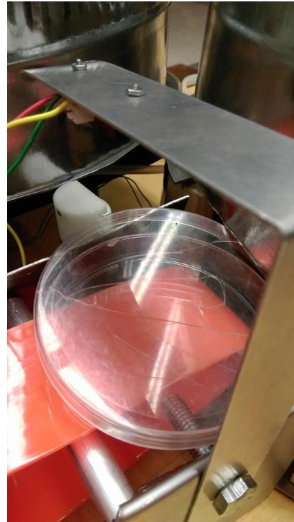
Figure 8: The rail has lifted the lid of the petri dish high enough for the proximity sensor to stop the conveyor belt and start the pinch valve sending agar solution into the opening. (above)
