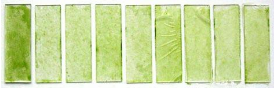
Figure 2-24. Typical growth of Ulva sporelings on amphiphilic coatings after 10 days.
