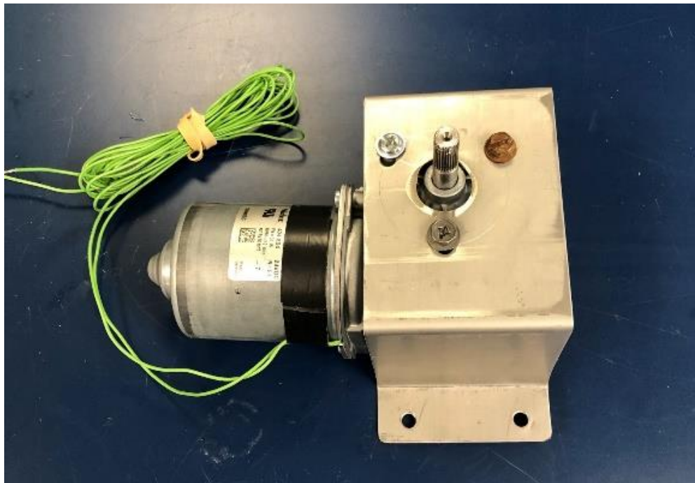
Figure 20: Motor with Mounting Bracket Top View
