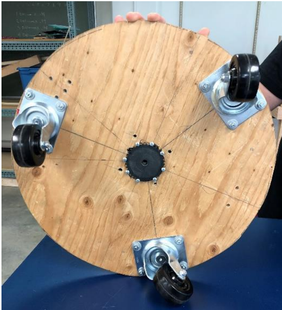
Figure 21: Rotating Platform Bottom View
