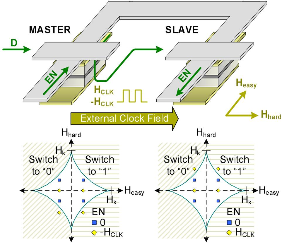
Figure 2: Enabled master-slave flip-flop constructed using two magnetologic latches. The  $D$  input is applied to the master latch, which is loaded when  $EN$  is active and  $CLK$  is low. When  $CLK$  goes high, the output of the master latch sets the value of the slave latch.
