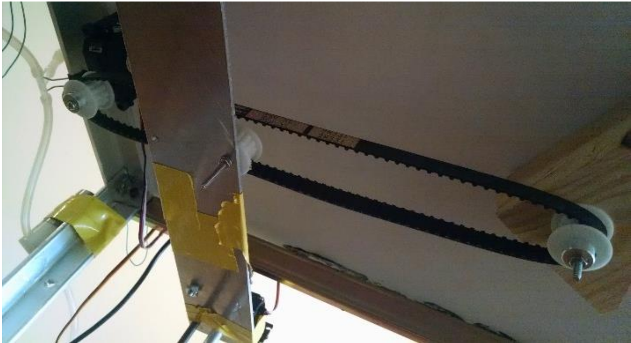
Figure 29: Final prototype pulley system (lower view)
