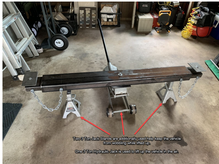
Fig. 14 Complete layout of the Cross Beam and additional equipment
