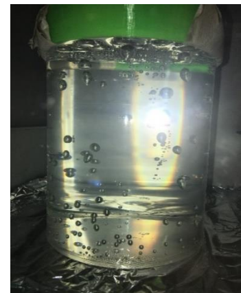
Figure 3: Degassing Sylgard 527 in a vacuum oven at 75 cm Hg for 4.5 hours. This picture was taken towards the beginning of the process.
