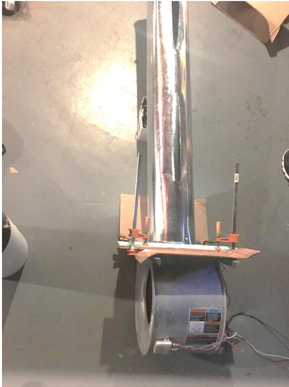
Figure 14: Initial balance testing of the rig with the side wall slots.
