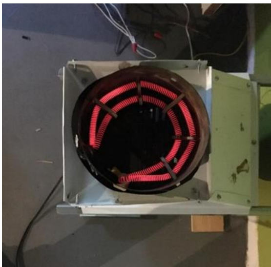
Figure 19: Nichrome resistive heating element before duct was attached to plenum.
