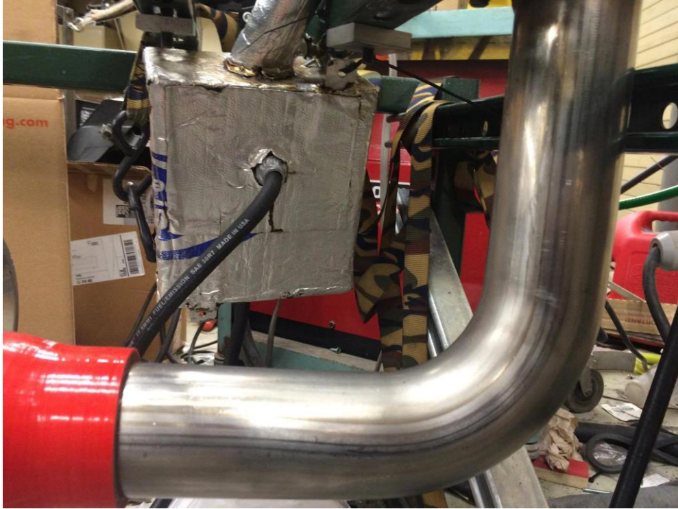
Figure 12: 90 degree Inlet into Combustion Chamber
