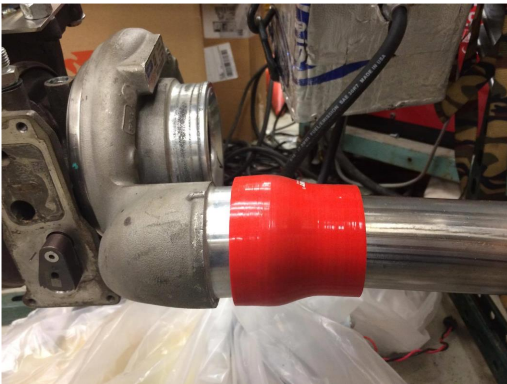
Figure 11: Connection between Turbocharger and Combustion Chamber Inlet
