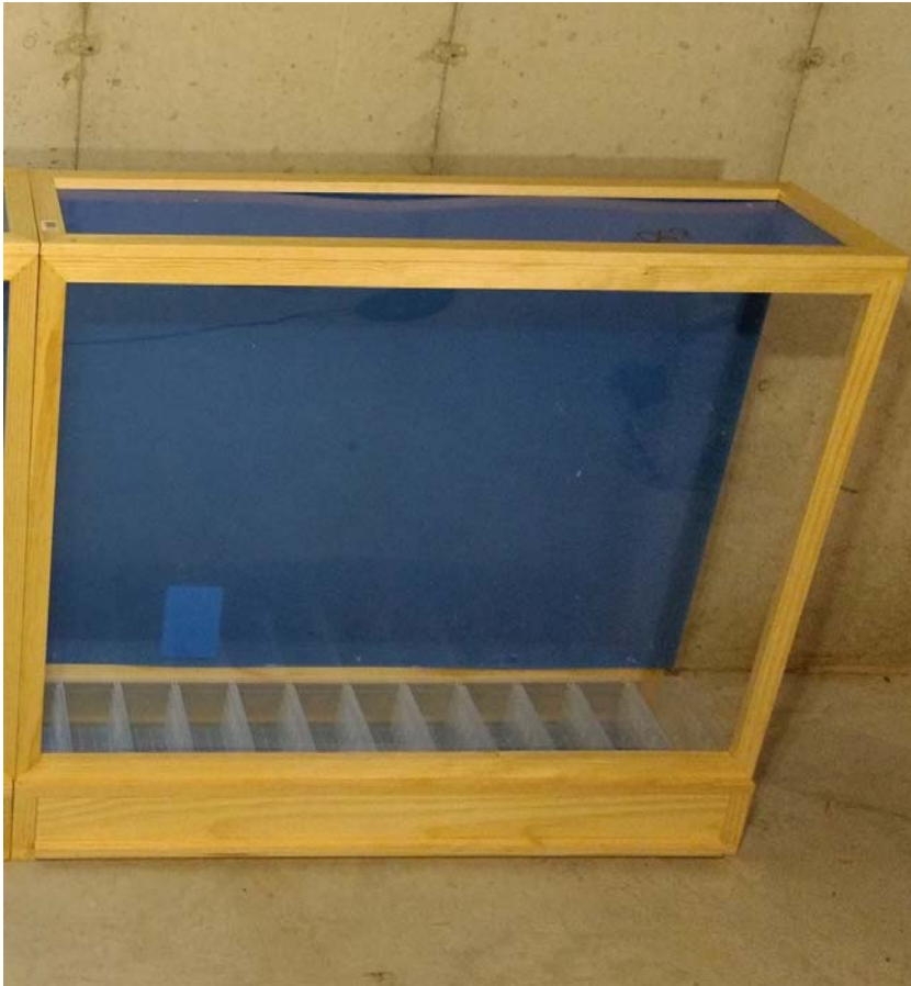
Figure 8.3.1 The Working Prototype's Tunnel Section.
