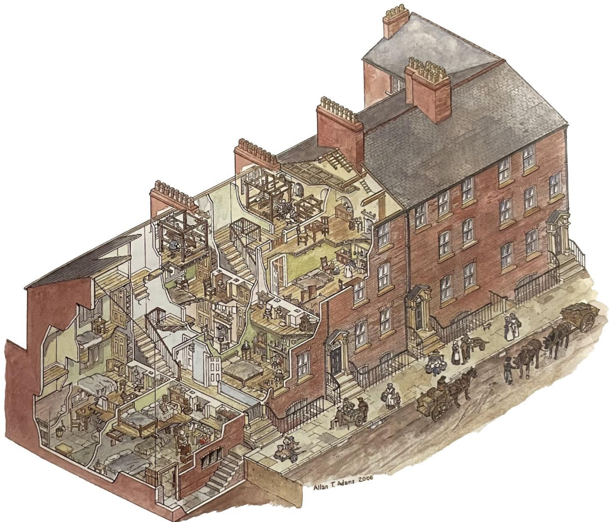
Figure 5: Reconstruction of Lever Street in the 1780s. Each floor was used as two-bedroom apartment or two single room apartments while the top floors functioned as workshop dwellings. (Taylor and Holder, 2008, page 25).
