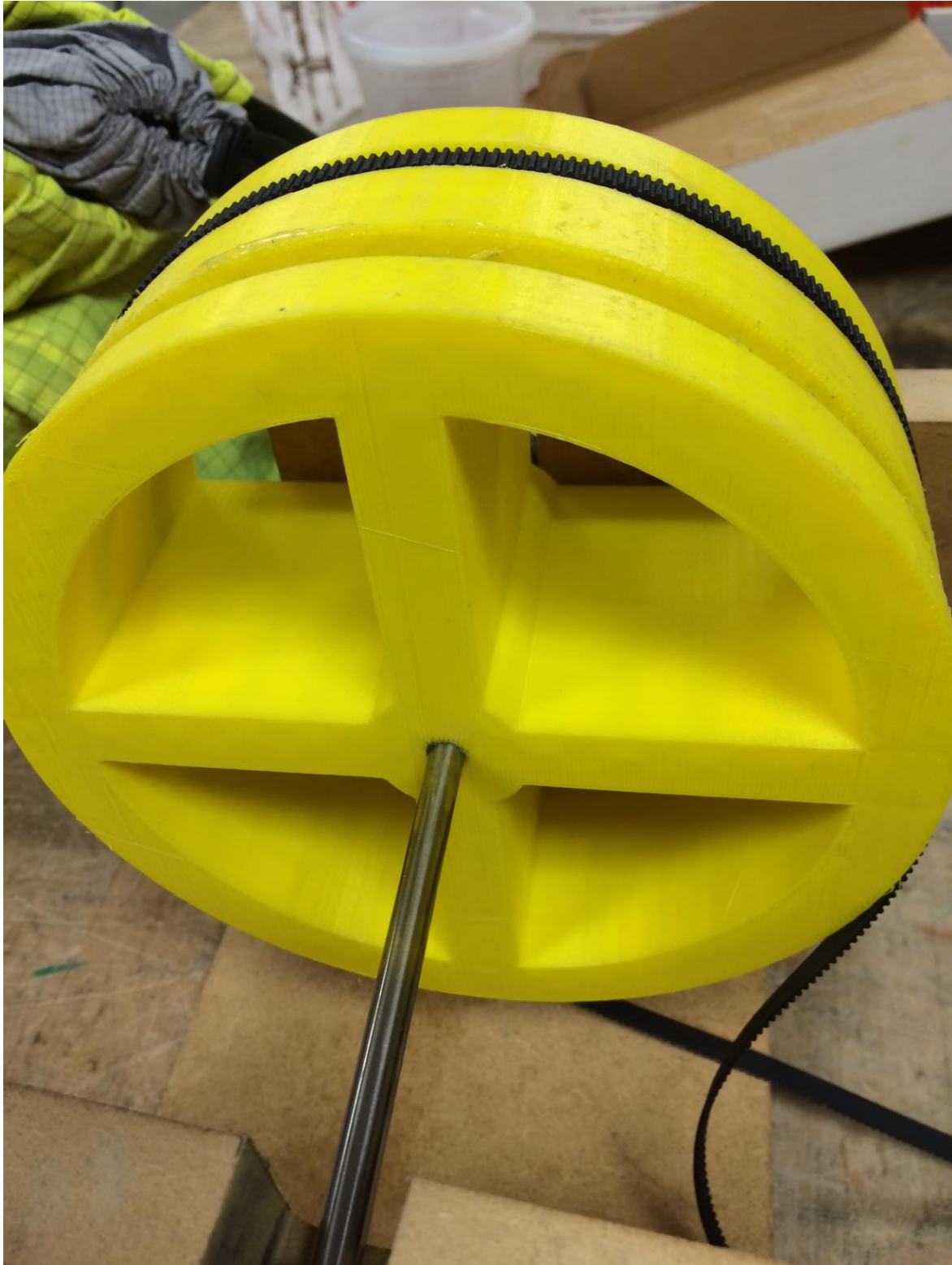
Figure 34: 3D Printed Cylinder (side view)
