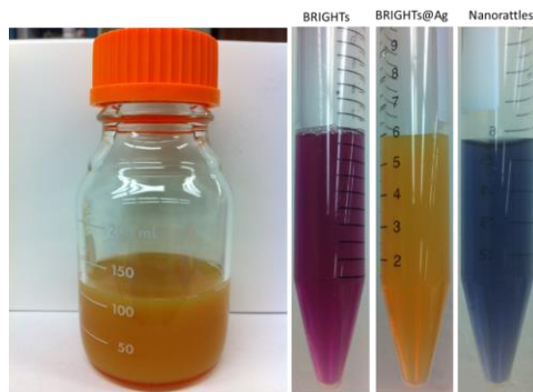
Figure S2 - Ag@BRIGHTs solution in a 200 ml bottle demonstrating the feasibility of large scale synthesis of the nanostructures and the solutions in centrifuge tubes exhibit the color of BRIGHTs, Ag@BRIGHTs, and nanorattles.
