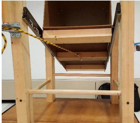
Figure 22: Chute support subsystem
