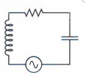
ter of a coil with symmetry axis aligned in the x-direction. To enhance the response, we connect the coil to a capacitor to create a resonant circuit with frequency equal to the precessional frequency of the proton.
