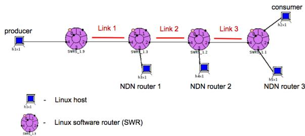
Figure 7: Mapping Topology onto Physical ONL Hardware
