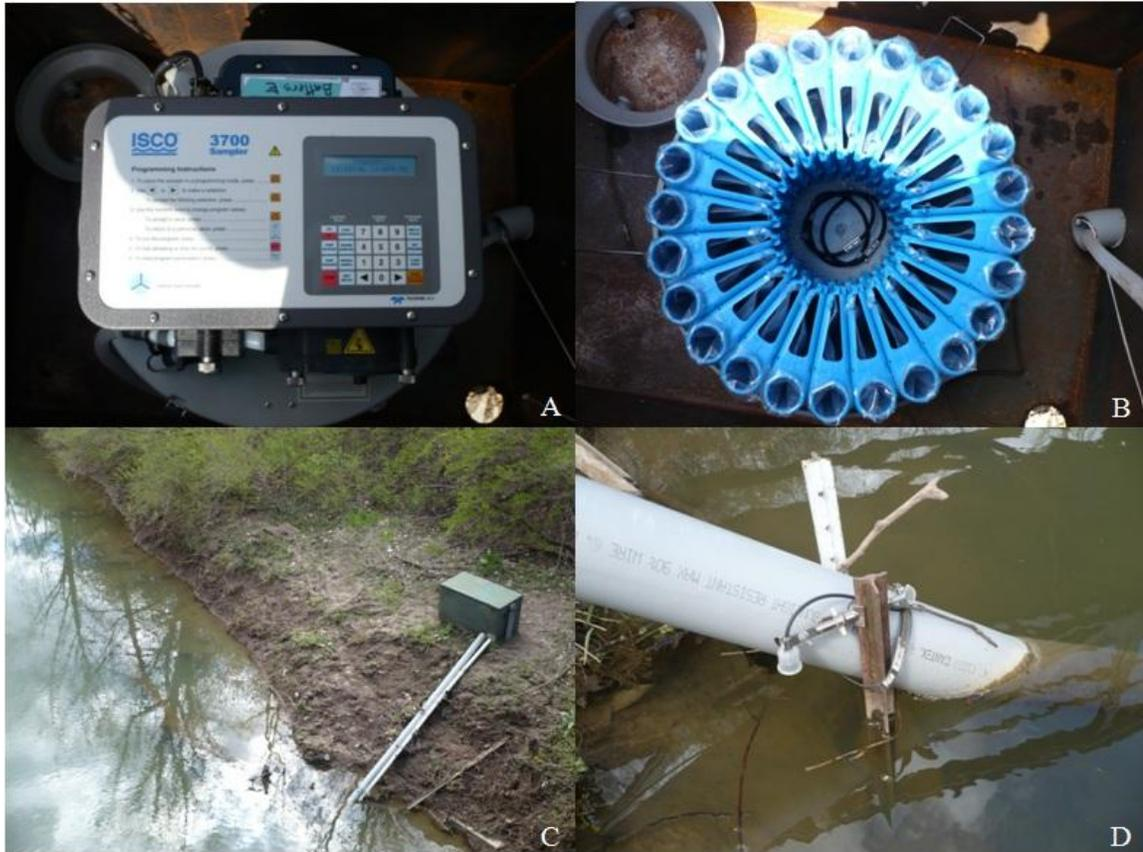
Figure 2.1. Typical autosampler field installation: (A) an ISCO Model 3700 autosampler; (B) a carousel filled with disposable ISCO ProPak™ bags; (C) the utility box and PVC pipe housing; and (D) the PVC pipe housing and the 1640 Liquid Level Sampler Actuator.
