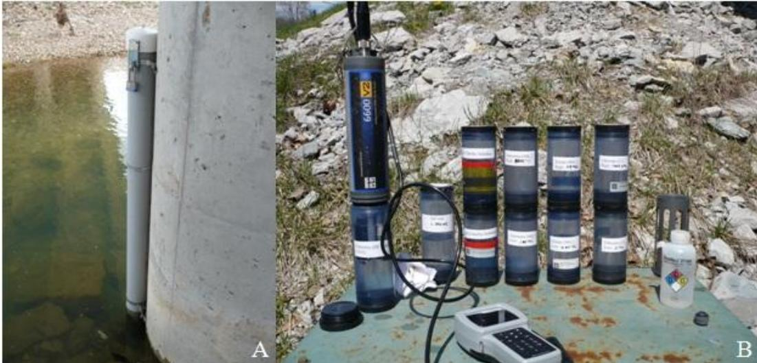
Figure 2.2. Typical in situ continuous water quality monitoring device field installation:
