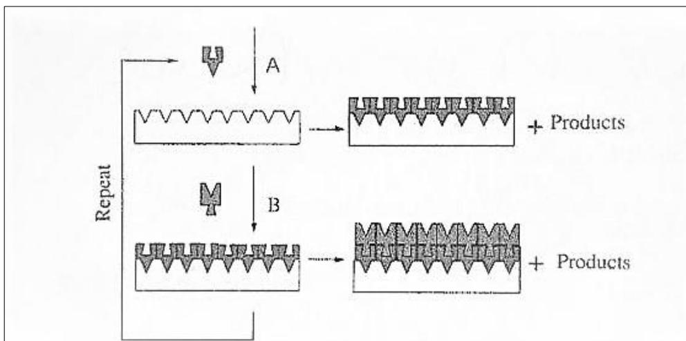
**Fig 1.** (op. cit. [2]) If we consider A to be the first gaseous substance, or precursor, it reacts with the surface substrate on a limited number of sites. Precursor B then undergoes a surface reaction with those sites, once again resulting in a finite number of new sites, with which precursor A will react. (Hence, the terms sequential and self-limiting) The final product of precursor A and B will be the binary compound desired.
