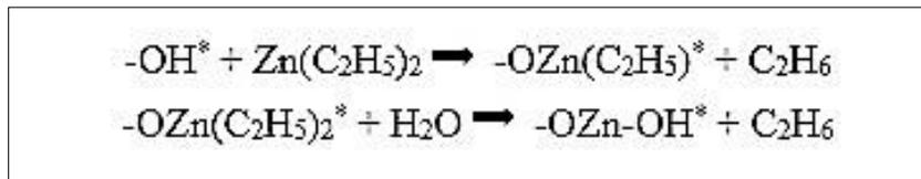
**Fig 2.** (op. cit. [3]) “\*” denotes a current surface site, “-” being the connection to the rest of the surface from the presented elements. The -OZn-OH\* is the equivalent of an -OH\*, with the -OZn added to simply demonstrate that a layer of ZnO has been added that terminates in an OH, allowing the cycle to start all over again.
